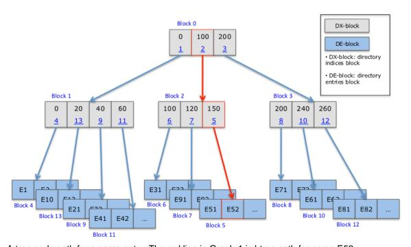
A tree node path for a name entry. The red line in Graph-1 is htree path for name E52.
