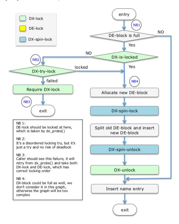
If the DX-block is full or the tree is full and needs to grow, we just need to lock the whole htree with EX mode and repeat the process of  $dx_probe()$  and  $dx_add_entry()$ .
