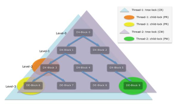
Two types of locking operation are available: tree-lock and child-lock. Graph-2 shows how they are used to protect htree directory.
